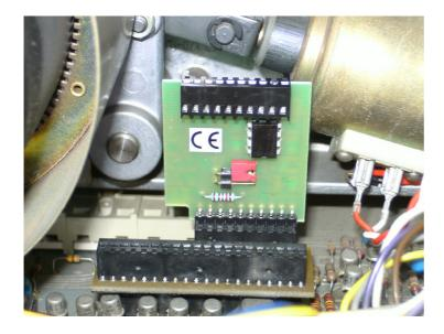
Carefully plug in the A700 connector board instead with plugged-in Pause Memory
