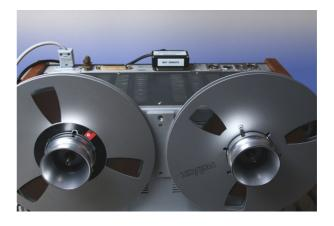
If you want to use the speed control facility on the B67 and need to have access to the speed connector it would be possible to produce the interface to your wishes – specially built with a rotated remote connector in an interface box to enable both remote and speed control.
